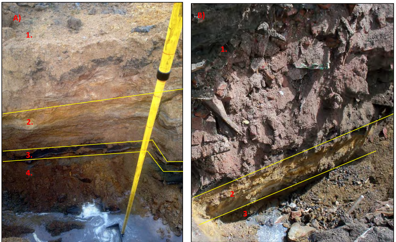
Figure 4A and 4B. Four lithologic units were observed above the water table in test pits; fill (unit 1), tailings (unit 2), black organic silt (unit A-3), and medium gray alluvial sand (units A-4 and B-3). Sediments were classified as fill material if they were found overlying tailings, and ranged from topsoil and fine-medium sand (A4) to landfill material (B4). Except for a few surficial deposits, tailings material in the Diggings East (A-2 & B-2) were typically encountered underlying 1-8 feet of fill material. The black organic silt layer (A-3) was observed at most-but not all-of the sites, and was encountered underlying the tailings and ranged from 0.5 feet to greater than 5 feet thick.
